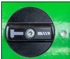
Drill symbol on mark - drilling without soft impact
